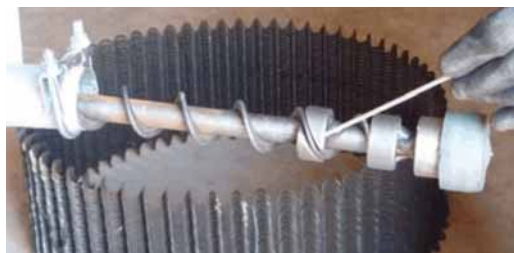
Figure 6-7 : Fixer la vis spirale
